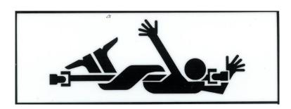
Never use your hands to clear if clogged. Never allow anyone to reach into the rotor housing. The rotor can crush and/or dismember. Keep everyone clear of the rotor until the prime mover engine is off and the hydraulic pressure has been relieved.
